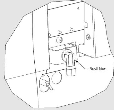
Remove Orifice from 90 degree fitting and replace with orifice from bag labeled IR Broiler Orifice.
